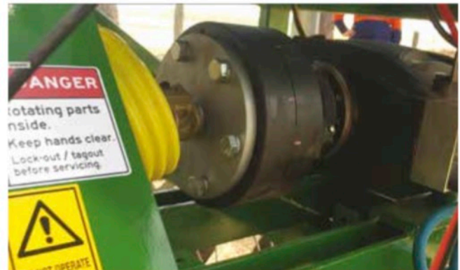
A torque clutch is a very safe way manage the interface between the tractor PTO and the Flow ultra-high-pressure pump.
