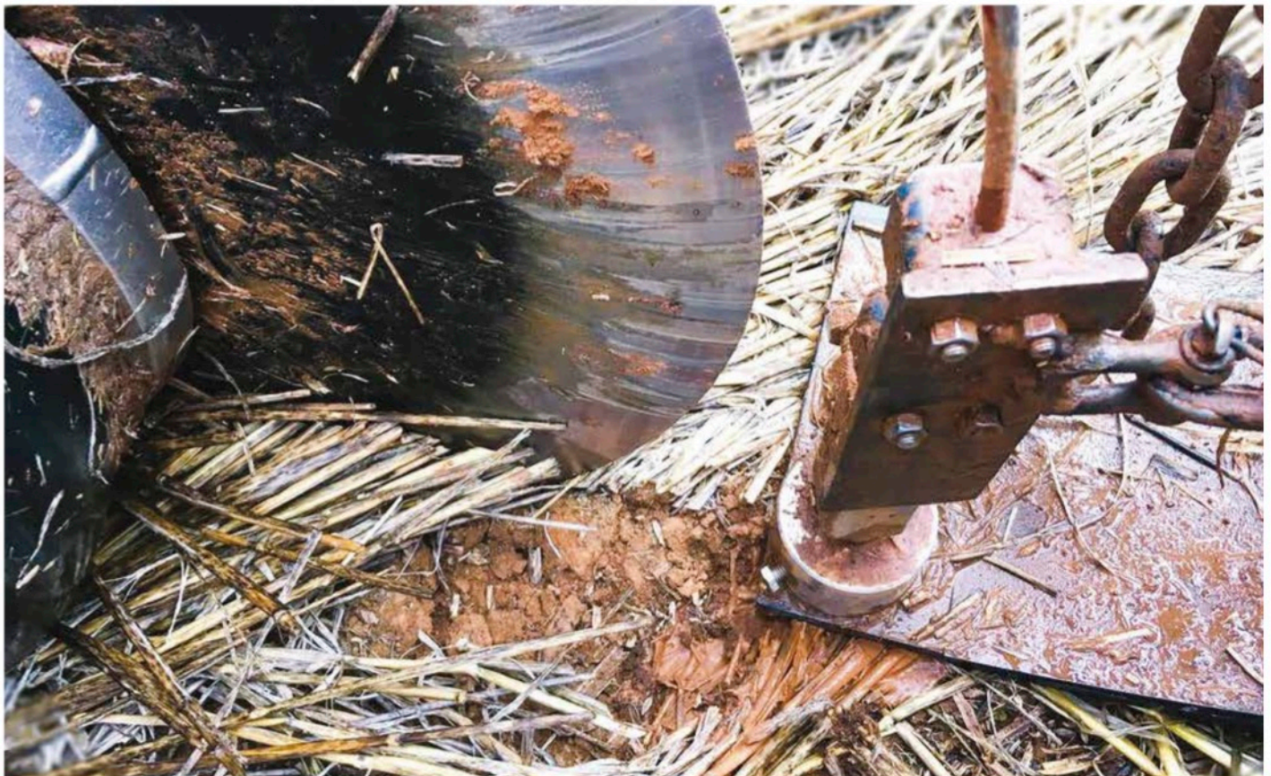
Ultra-high-pressure liquid deployed through a ski can be used as a clean cutting coulters in a process known as AquaTill.
