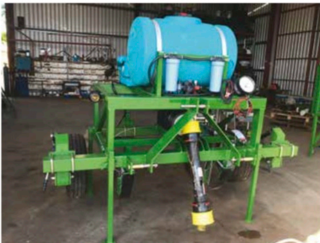
Seabrook Seeders integrated a Flow ultra-high-pressure pump into a 2 Nozzle AquaTill trial machine especially designed for sugarcane experiments.
